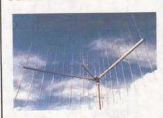
In the overall scheme of things, corner reflectors have a spot in the logical progression of antenna evolution. The ordinary dipole gave way to the Yagi-Uda, which utilized directors and a reflector. The single reflector was turned into a screen for a greater back-side rejection. The screen (Continued on Page 4)
